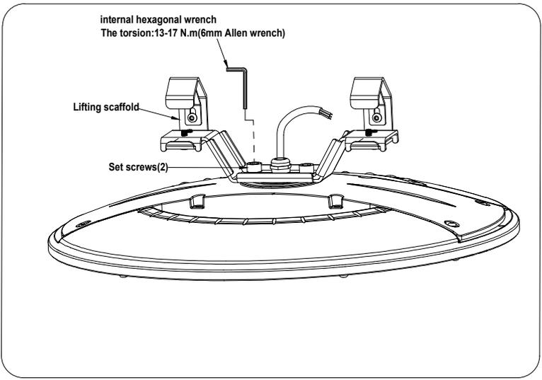
**Step 2: The lifting bracket is fixed on the lamp body and then hung on the wire rope.**
