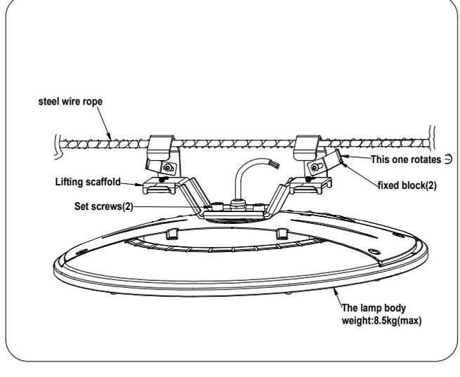
Step 3: pass the wire rope through the lifting bracket, adjust the position of the fixing block, and tighten the screws with the hex wrench to fix the position
